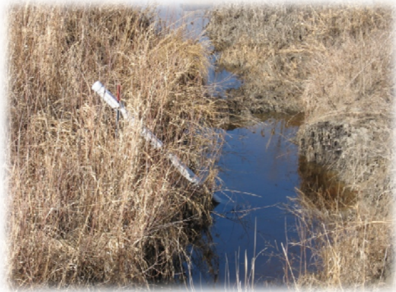
Figure 8. HOBO Water Level Logger deployment pipe installed in CD1, west of Crookston
