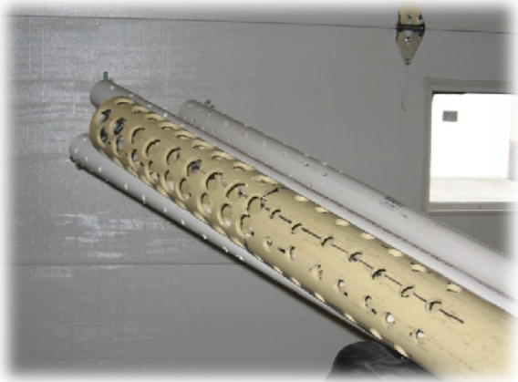
Figure 5. Sonde and Water Level Logger pipes, ready to be installed.
