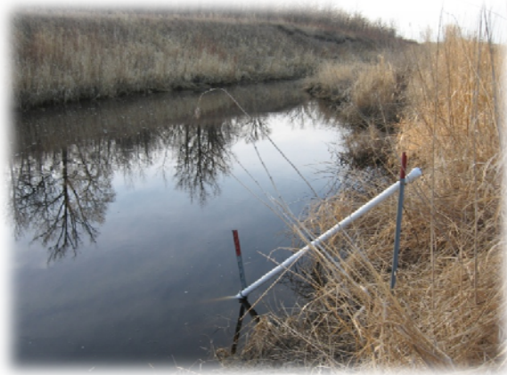
Figure 9. HOBO Water Level Logger deployment pipe installed in JD60, east of Crookston
