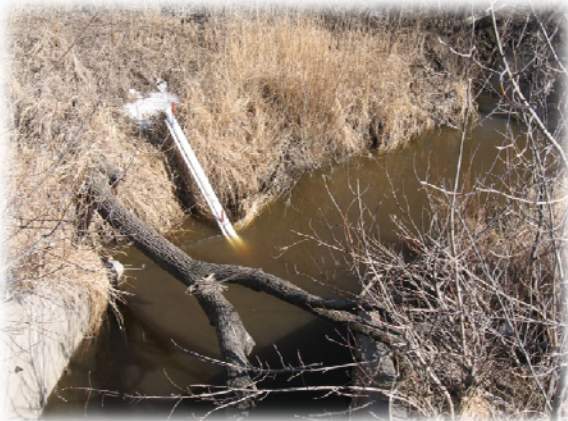
Figure 6. Eureka Midge and HOBO Water Level Logger deployment pipes installed in Kripple Creek
